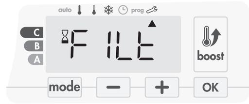
Before any action of filter removal, switch off the device by pressing the button located under the blower.
