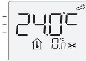
Decrease the temperature measured by the ambient temperature sensor by 2°C by pressing **-**.
