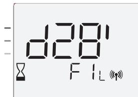
The blower continues to operate but does not heat up. If the controller is a blower, check if nothing is put in front of the ventilation grid to not block the air flow. The filter could be plug by dust, it must be cleaned.
