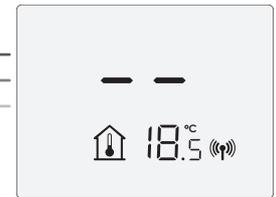
To exit standby mode, press the standby button.
