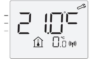
Increase the temperature measured by the ambient temperature sensor by 2°C by pressing **+**.
