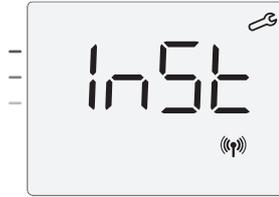
4- Press and hold **+** and **OK** simultaneous for 10 seconds.
